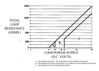
Please consult with the installation/service manual that was provided with your receiver for specific wiring instructions. Most Anderson receiver (displays, chart recorders, etc.) are capable of supplying loop power. Typical wiring would be as shown on following page.
