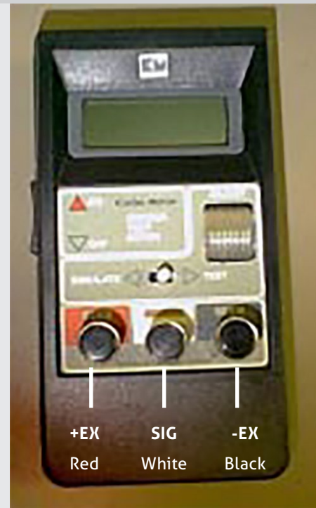
Figure 2-1 Anderson-Negele Test Meter
