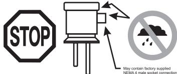
Be sure to keep moisture from entering the probe housing prior to completing field installation and startup. Upon installation, be sure no moisture path exists into housing.
