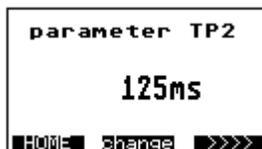
By means of the key **change** the pulse length of TP2 in ms can be changed for output IMP2. TP1 is valid for Mode1 & 5 only. The value of 0 ms is used to set the pulse-to-pause ratio to 1:1. You might be prompted to first input an unlock code.
