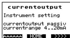
On this image level the settings for the current output are made.
