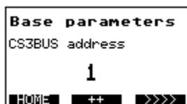
The CS3-Bus address can be changed by means of the key **++**. You might be prompted to first input an unlock code.
