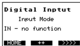
The function of the digital input can be selected by means of key **++**.
