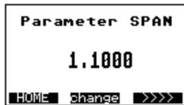
The SPAN value can be changed by the aid of the **change** key.
