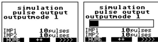
This simulation can be used for checking a cable connection or a counting instrument or even a connected controller. According to the output mode, the number of pulses to be simulated is shown in display lines 6 and 7. The simulation is started by the key **++** and a bargraph is displayed. The simulation is finished when the bargraph is completely filled. Then the bargraph is erased.
