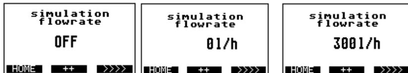
This function can simulate the complete metrological functionality of the IZMAG™ converter, i.e. the pulse outputs and the current output behave like in the normal operation. This function is suitable for the “dry” commissioning of a system or of system sections.
