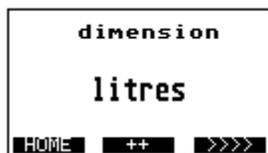
The **++** key can be used for changing the dimension (unit) of the measured value. You might be prompted to first input an unlock code.
