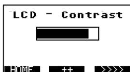
The LCD contrast on the flow meter's display can be increased by means of the key "++", continuing to use the "++" key will result cycle past the highest available contrast back to the lowest contrast.
