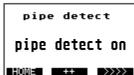
The empty pipe detection can be switched on and off by means of the **++** key.
