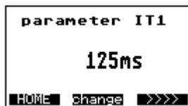
The **change** key can be used to change IT1 to ms. IT1 determines how long the signal will have to be available for the input to permit the selected function to become active.
