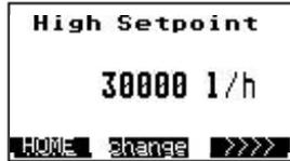
Defines the High threshold flow rate value for IMP2. Only applicable when Mode 31 is in use.
