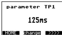
Use the key **change** to change the pulse length of TP1 to ms. TP1 is valid for Mode1 & 5 only. The value of 0 ms sets the pulse-to-pause ratio to 1:1. You might be prompted to first input an unlock code.
