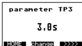
By means of the key **change** you can change the time delay TP3.
