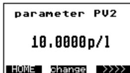
The key **change** can be used to change the pulse value PV2 for the output IMP2. PV2 is valid for Mode1 and mode 5. You might be prompted to first input an unlock code.
