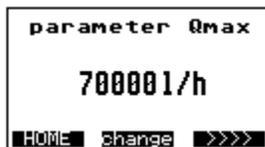
The key **change** can be activated for changing the Qmax value for the current output.
