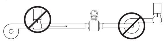
Warning: Before welding on a pipline with a flowmeter installed, unplug the flowtube cable from the meter
