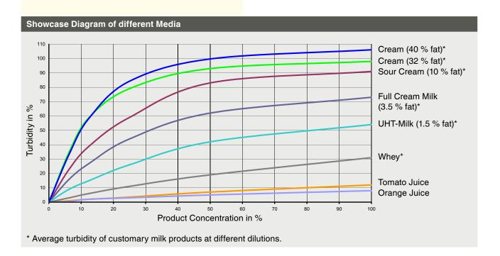
Depending on particle form and size, the slope of the characteristic curve is decreasing while turbidity is increasing. This is primarily caused by dampening/absorption effects due to multiple reflections inside the media. The turbidity measured in the production process can deviate from the graphs shown above, depending on product, process step and production process.
