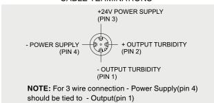
M12 PLUG-IN RIGHT SWITCHING OUTPUT RANGE CONTROL VOLTAGE CABLE TERMINATIONS
