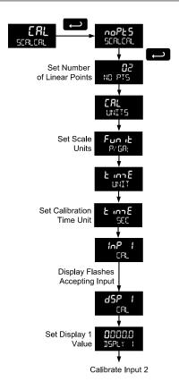
The multi-point linearization feature (nopts) can be used to linearize the display for non-linear signals. For instructions on how to utilize this feature, see Multi-Point Linearization (nopts), page 44.
