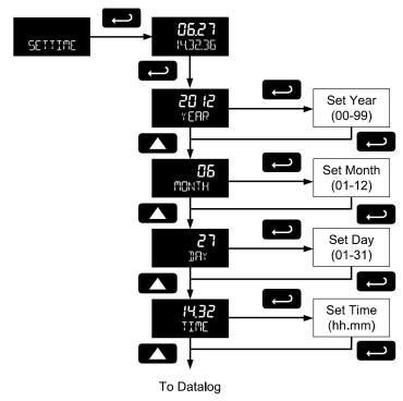
The year, month, day, hour, and minute may all be set by the user. The real time clock will need to be reset if external power and battery power are lost. Changing the time (hours and minutes) will reset the seconds clock to 0.
