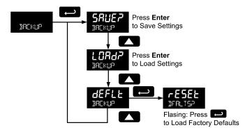
The save feature (SAvE?) saves all current parameter settings into the memory of the backup restore. The backup restore feature is loaded with factory default settings until a new configuration is saved.
