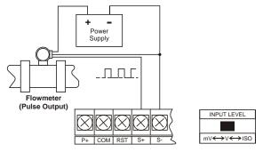
Figure 2. Flowmeter Powered by External Supply (Active)
