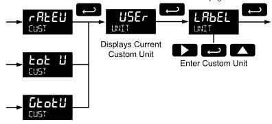
Fully alphanumeric values are set using the **Right** button to select the digit to be changed. Press the **Up** button to begin editing the digit, then the **Up** and **Right** arrow buttons to select the next or previous alphanumeric character. Press the **Enter** button to confirm and select the next digit to change. For details on setting alphanumeric labels, refer to Setting Alphanumeric Labels (LABEL) on page 17.
