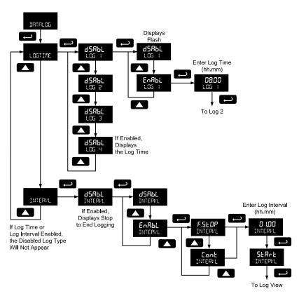
There are two ways to configure the time when a data log is recorded. The Log Time feature allows up to 4 data logs to be recorded each day, at specific times. The Log Interval feature allows a data log to be recorded each time a time interval has passed.
