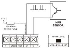
Figure 5. NPN Open Collector Input (NPN)
