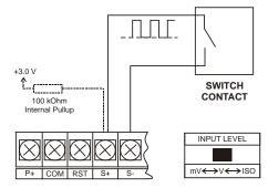
Figure 7. Switch Contact Input (Reed)
