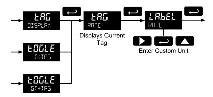
Fully alphanumeric values are set using the **Right** button to select the digit, the **Up** and **Right** arrow buttons to select the digit reading, and the **Enter** button to confirm and select the next digit.
