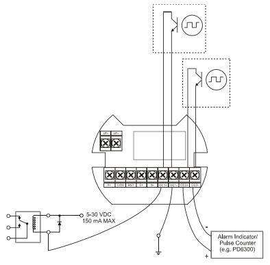
Figure 10. Open Collector Output Connections
