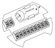
Figure 11. Battery Orientation
