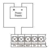
Figure 8. DC Power Connections
