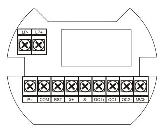
Figure 1. Connector Board
