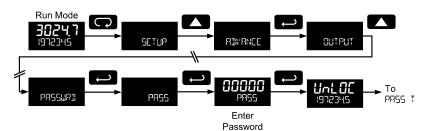
If the correct five-digit password is entered, the meter displays the message UnIOC (unlocked) and the protection is disabled until a new password is programmed.
