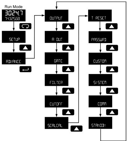
Advanced menus A OUT displayed only for meters with the analog output option, COMM displayed only for meters with the serial communications option, and STANDBY only for meters with battery or battery backup power.
