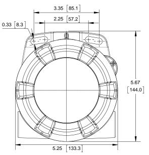
Figure 13. Enclosure Dimensions – Front View
