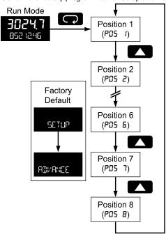
To add a menu or parameter to the menu structure, or change the default menus, press **Enter** at the desired menu in the position (POS) to be edited, and use the **Up** or **Right** arrows to select the desired menu item for that position. See page 50 for a complete list of the available menu selections for each position.
