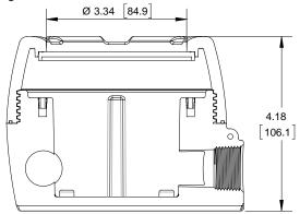
Figure 14. Enclosure Dimensions – Side Cross Section View
