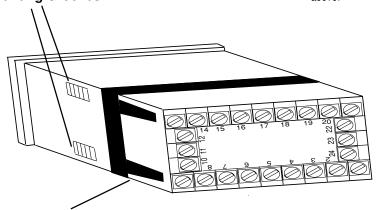
gasket is not distorted and the instrument is positioned squarely against the panel. Slide the mounting clamp into place on the instrument, as shown to the left, and push it forward until it is firmly in contact with the rear face of the mounting panel and the tabs on the bracket arm are seated in the mounting grooves on the side of the unit.
