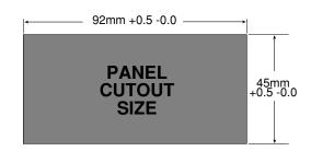
should be made based on the recommended panel opening illustrated in the drawing above.
