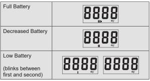
NOTE: When removing batteries, wait a minimum of (2) two minutes before re-installing.
