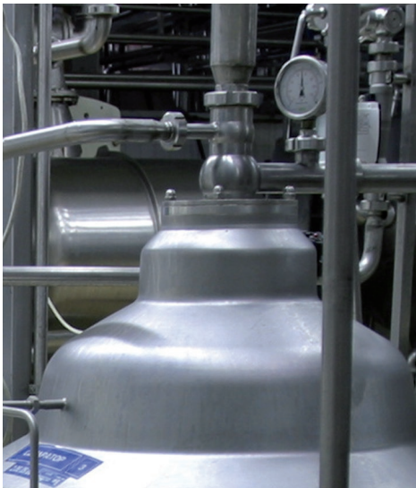
Compact pressure gauge with hygienic process adaptation CLEANadapt 63 mm
