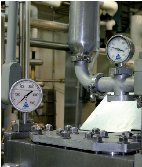
Pressure gauge with integrated transmitter for homogenizers
