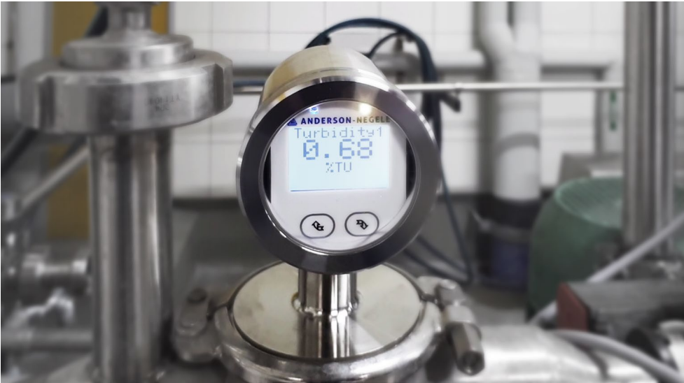
Turbidity sensor (backscatter light) in modular design
