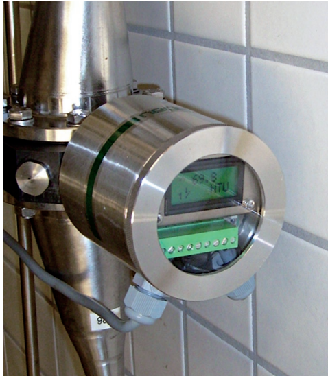
Turbidity sensor (4-beam alternating light)
