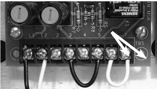
4. Make sure Run/Program jumper is in the Run position.
