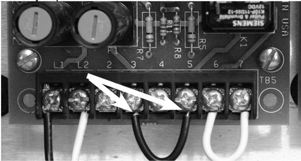
3. Install a second jumper wire from terminal 6 to terminal 7.
