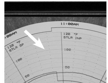
7. Expose HTST probe to a temperature above diversion setpoint – The forward flow (green) light should be on and the event line at the outside edge of the chart should be recording at the outer (forward flow) position.
