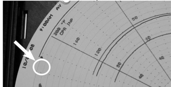
6. Expose HTST probe to a temperature below diversion setpoint – The divert flow (red) light should be on and the event line at the outside edge of the chart should be recording at the inner (divert) position.
