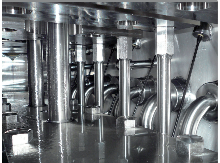
Fig. 4: NVS limit switches in the metering device
