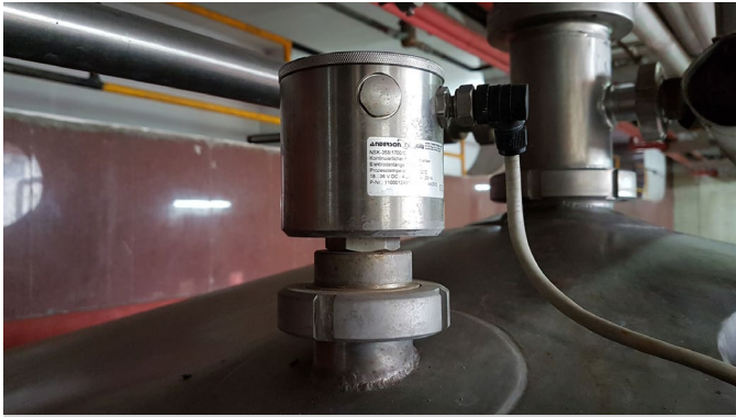
NSL-F on top in Flash Pasteurizer Tank
