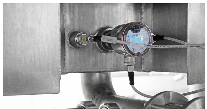
The standard equipment for process vessels: Temperature (TS), Level (L3) and Point Level (LS)
