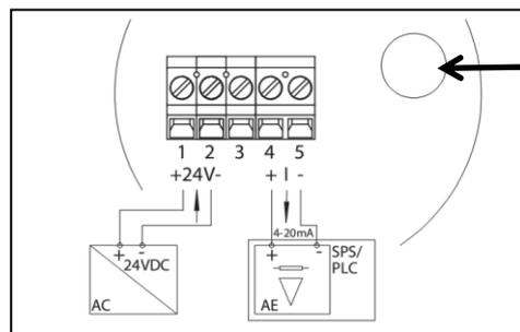
Connection plug for MPI-200-F adapter as an intermediate plug between the NSL-F electronics and the MPI-200 connection 3 (see next figure).
