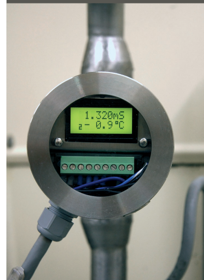
Figure 2: Continuous conductivity measurement at the reaction tank with inductive conductivity meter ILM-2 from NEGELE
